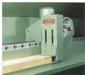
The cut at the end of the work piece can be made at any point (down to waste "Zero") along the remaining waste piece, as the clamping device is released and withdrawn before sawing.
