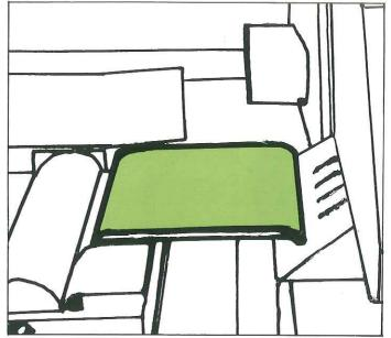
As soon as the work piece is fixed by the clamping device and fed towards the cross-cut saw, leaving the slide bench vacant, the operator can put on the next work piece. The advantage: the operator need not wait for the return stroke of the limit stop but can place the next work piece on the slide bench as soon as it is vacant. The effect is a greater capacity.
