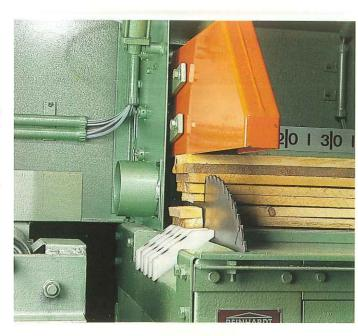
The work pieces can be placed on top of or beside each There is an optional extra clean cut which is exother. This increases the capacity of the machine enor-ecuted automatically. mously.
